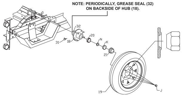
Figure H: Hub/Wheel Assembly
